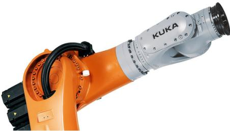
A photograph of a KUKA KR 240 R3330 F robotic arm. The arm is orange and grey, with the KUKA logo visible on the upper arm. It is shown from a side-on perspective, slightly angled, with its end effector pointing towards the top right. |
